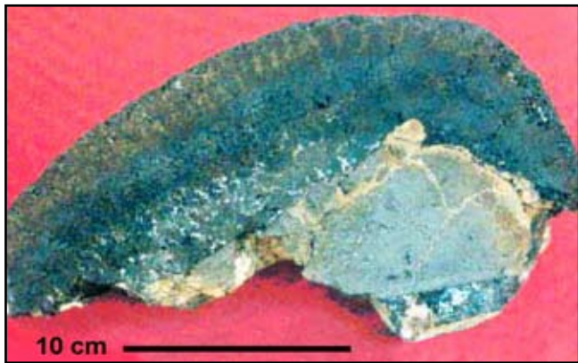
A dark cobalt-ferromanganese crust revealed in a cut section (source: CoRMC-H, Auki).
