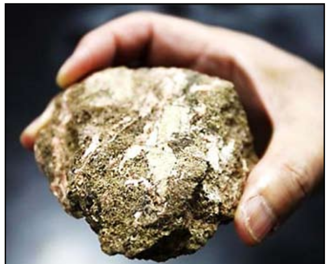
Sample of the carbonate-fluorite mineral bastnaesite that contains rare earth elements; at the laboratory of Yasuhiro Kato, Tokyo University (photo: Reuters, Yuriko Nakao, 2011).
